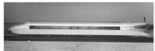
This prototype high-speed train travelled at 230 km per hour from Hamburg to Berlin, 1931. It was built by the Krukenberg engineering company.
