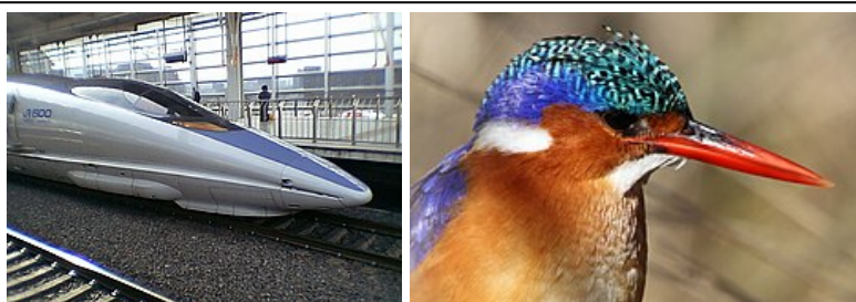
The streamlined design of Shinkansen 500 Series (left) mimics the beak of a Kingfisher bird (right) to improve aerodynamics.
