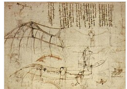
Leonardo da Vinci's design for a flying machine with wings based closely upon the structure of bat wings
