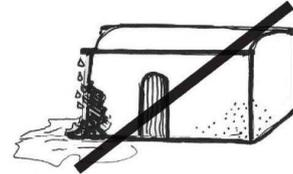
Ensure that the surrounding ground is clear so that rain does not damage the wall base
