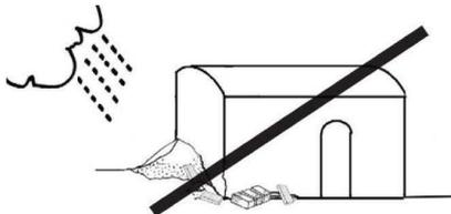
It is essential to infill and buttress the vault to ensure its stability
